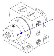
If the pump is installed in any kind of locked space (boards, cabinets, etc.), the cold air mustn't be halted behind the muffler.
